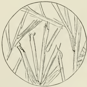
Crystals of Acetate of Lead, magnified 80 diameters.
